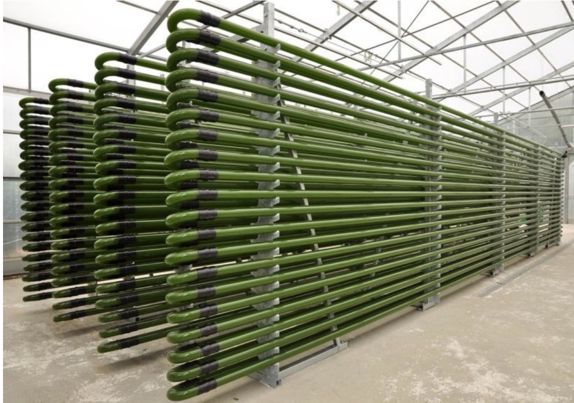
A photobioreactor for algae. https://commons.wikimedia.org/wiki/File:Photobioreactor_PBR_4000_G_IGV_Biotech.jpg
